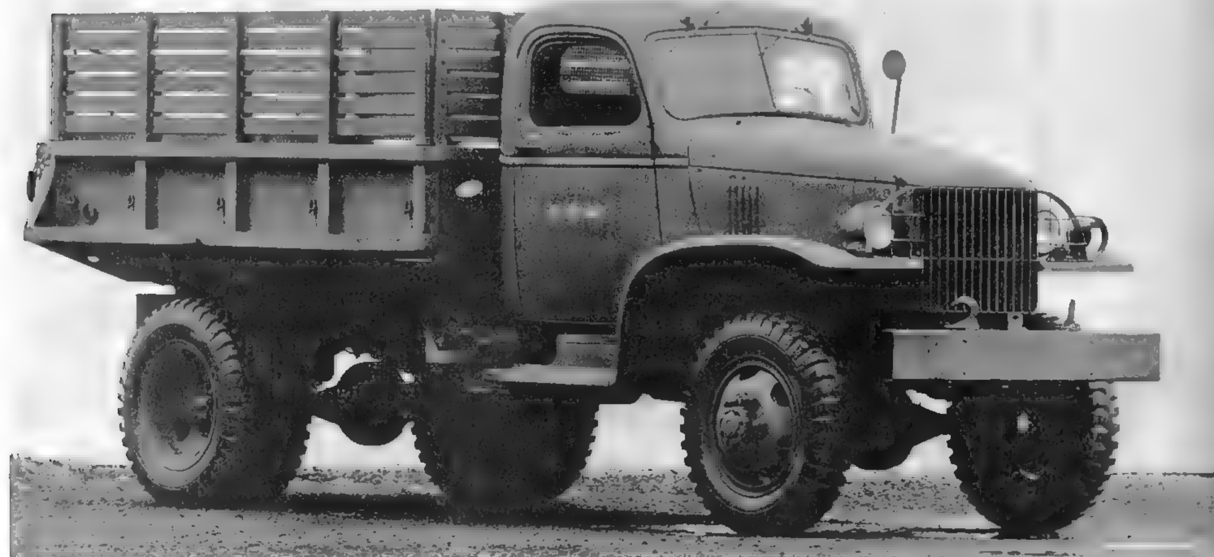
This November 1944 photo taken at the Studebaker Proving Ground shows the typical 1 1/2-ton Chevy G7107. This particular truck has a steel bed. The liquid container bracket can be seen beneath the fuel filler. (U.S. Army photo)
